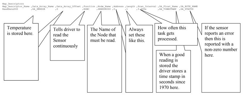
This Configuration Fragment Illustrates a configuration to read 3 sensors. If the module is offline then the bit corresponding to the Node\_ID in the Data Array named DA\_Node\_Status will be set to zero (online=1). If the sensor responds with an error then the driver will overwrite the value stored in DA\_Sensor with 999.9.
